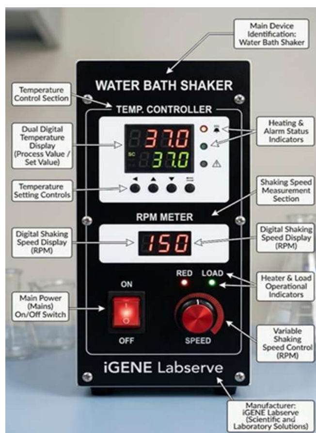
Figure 7. Close-up of a digital control panel featuring dual LED displays for Temperature and RPM control, similar to the iGene Labserve model
