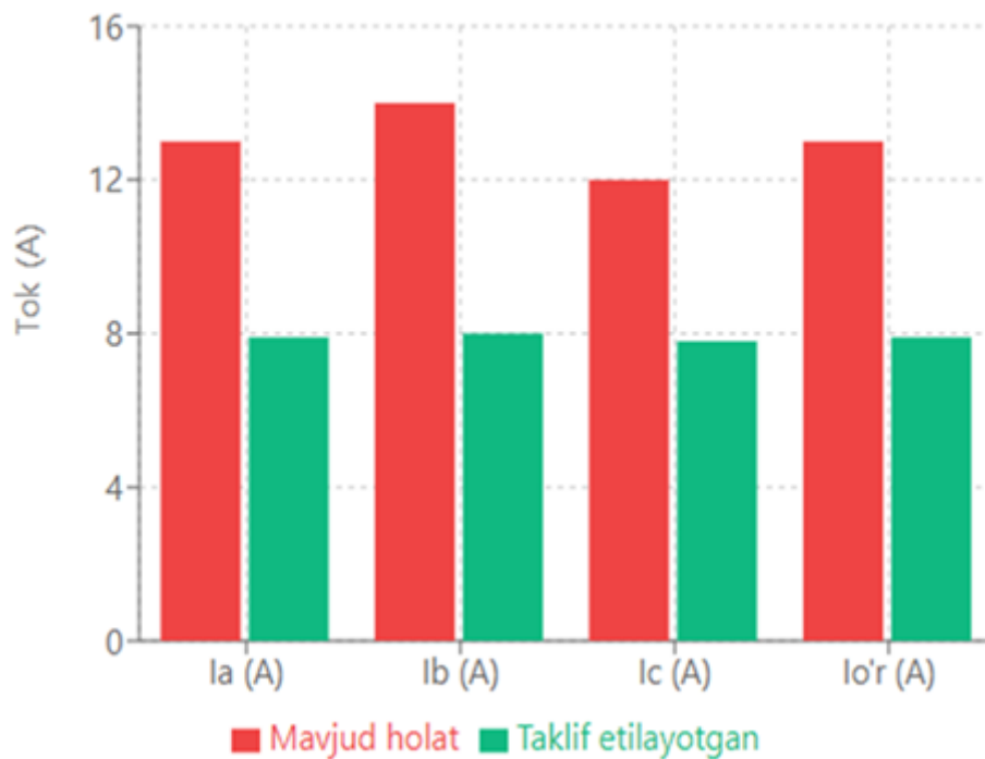
Figure 1. Comparison of current parameters for lint removal during single gin operation under load
